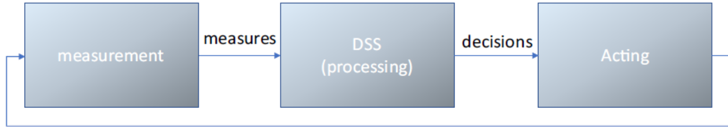
FIGURE 1.4 The decision support system process.
