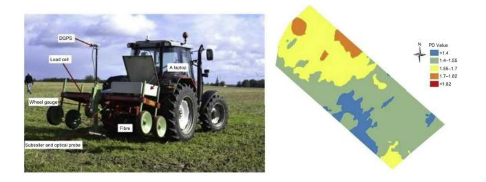
Online soil sensor (left) and packing density (PD) map (right). The three PD classes on the map have been merged into three tillage zones as described in the text.
