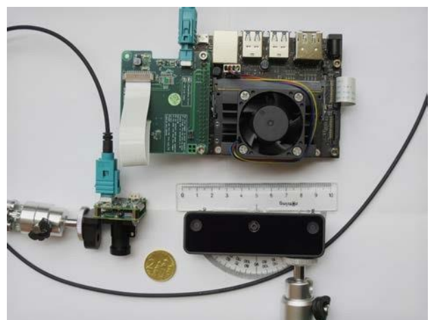
Fig. 1: Jetson Nano [5] with camera extension board and coaxial cable, in comparison to OAK-D lite [6], which integrates three cameras and processing board in a single case.
