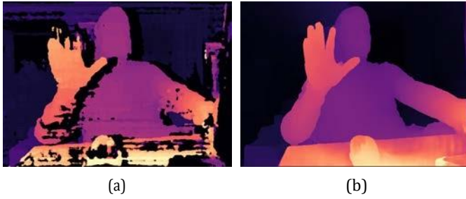
Fig. 4: Visual comparison of performed stereo depth perception experiments: (a) 'on device' solution based on [6]; (b) 'on host' solution based on method from [33] and the same image pair.
